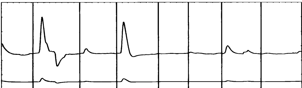
FIG. 7—Identical electrodermal reactions on different scales. The vertical lines indicate the beginning of the question.
